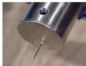
Fig 4: Special micro-Pitot probe used to characterize boundary layers
