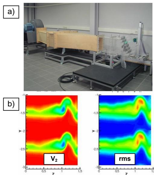
Figure 1: a) General view of the low-speed linear cascade with LDV system. b) Secondary flow characterization.
